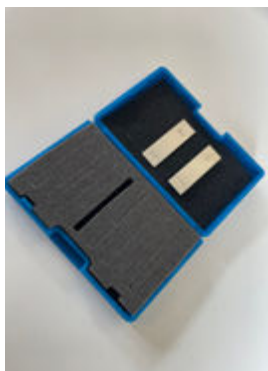
Traceable 2000 µm and 500 µm checking gauges
