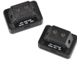
Certified high and low gloss calibration tiles
