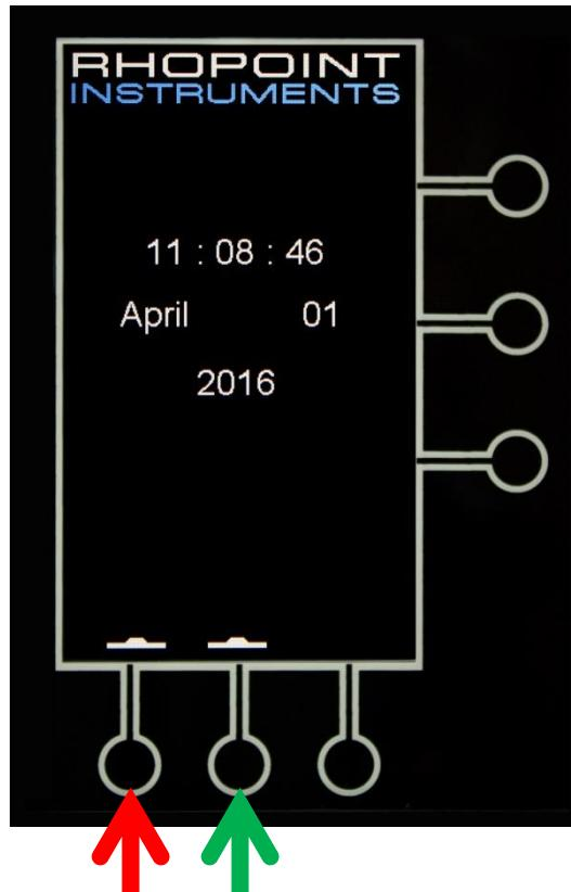
Press the button marked with a green arrow to start adjusting the time and date. This will enable up and down arrows on the right hand side of the screen. Pressing the up and down arrows will change the highlighted field. Pressing the button with the green arrow will move to the next field. Pressing the button with the red arrow will save the changes and exit the menu.
