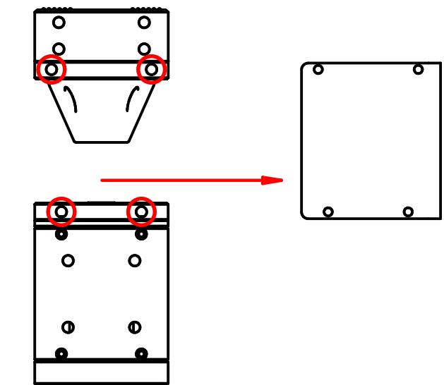
Ensure that you Remove the spacer in the correct Direction
