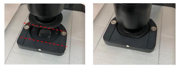
Take a reading on the checking standard by pressing the tick icon and compare the result with its assigned value. The value must match the assigned value within the tolerances printed on the label.
