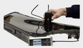
The Rhopoint IQ Flex 20 quantifies surface quality problems such as orange peel and haze that are invisible to a standard glossmeter. It profiles how light is reflected from a surface.
