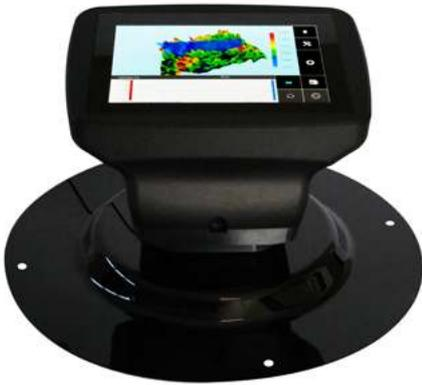
Its large measurement area (65 x 54mm) and speed of operation (under 10 secs) provides rapid measurement with results that are more representative than those made with profilometers or other optical scanning instruments and can be reported in traceable SI units or other industry specific units.
