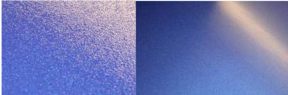
An example of test panel with low and high DOI values. Orange peel, texture, flow out and other key parameters can be assessed in coating applications where high gloss quality is becoming increasingly important.
