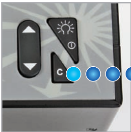
Press and HOLD the 'C' key to start calibration.
