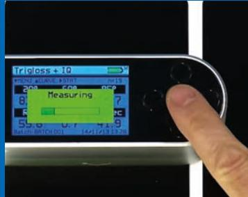
Single button push to initiate measurement of all parameters
