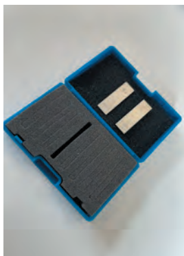
Traceable 2000 µm and 500 µm checking gauges
