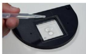
**STEP 2:** The two-piece accessory allows plastic film samples to be trapped within two optically clear glass slides mounted in the unit.
