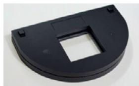
One half of the analysis plate without sample is mounted onto the Rhopoint ID and the unit tared.
