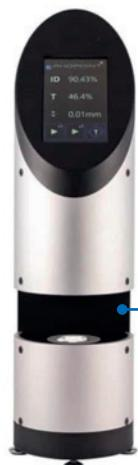
**STEP 3:** The analysis plate is placed into the Rhopoint ID measurement aperture and a measurement is taken.
