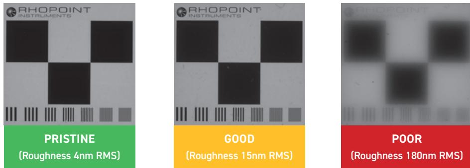
**STEP 1:** Three different samples of 0.25-mm-thick PMMA chemically etched film were used to simulate the effects of surface roughness. Each sample was tested using Rhopoint ID-L.
