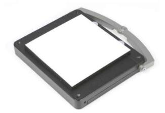
\* The sled has been calibrated to 200g including the magnet bars. If for any reason the magnet bars cannot be used to secure the sample use tape and then place the magnet bars on top.
