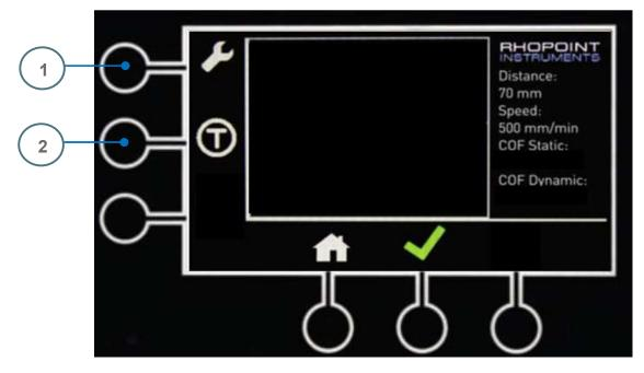
Ensure there is 0 load on the load cell. The sled should be removed from the instrument.
