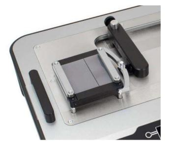
When in the home position menu press the **button** (2) again to move the load cell arm to the current home position setting. The load cell arm will move so ensure there are no obstructions such as the sled.
