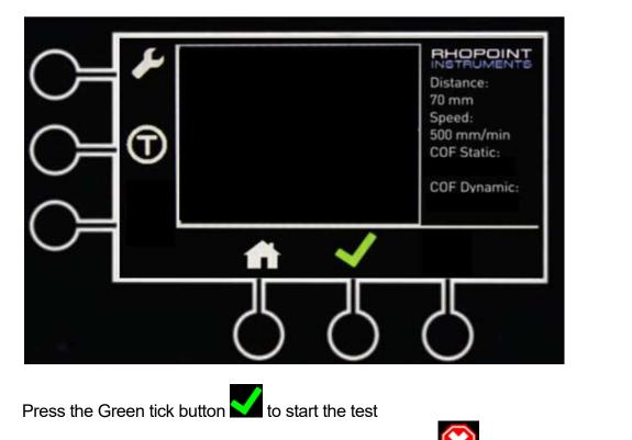
During the test run the emergency stop button is shown . Pressing this will abort the test.
