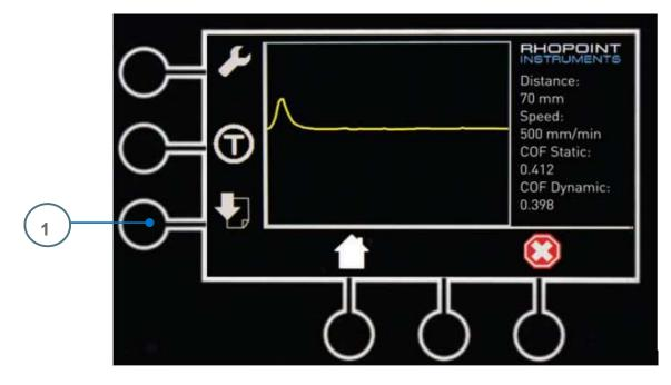
Once the export results button has been pressed the instrument will beep once to indicate a button press and again to indicate the export is complete. The USB stick can then be removed from the instrument and plugged into a PC device.
