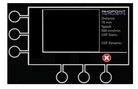
During the test a live reading from the load cell is shown on the graph. When the test has finished the graph will re-scale to maximize the graph display, please note that the scale is fixed after the first reading and is only an indication of test progress. The COF Static and COF Dynamic will be displayed bottom right of the screen.
