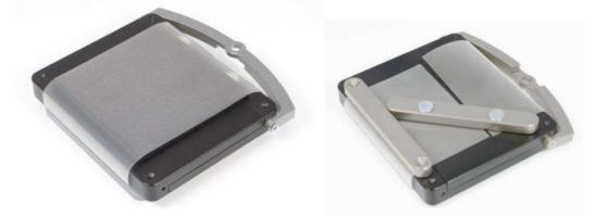
\* The sled has been calibrated to 200g including the magnet bars. If for any reason the magnet bars cannot be used to secure the sample use tape and then place the magnet bars on top.
