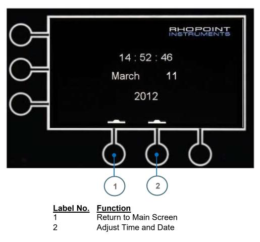
Press Button 2, the first field to be adjusted will be highlighted in green.
