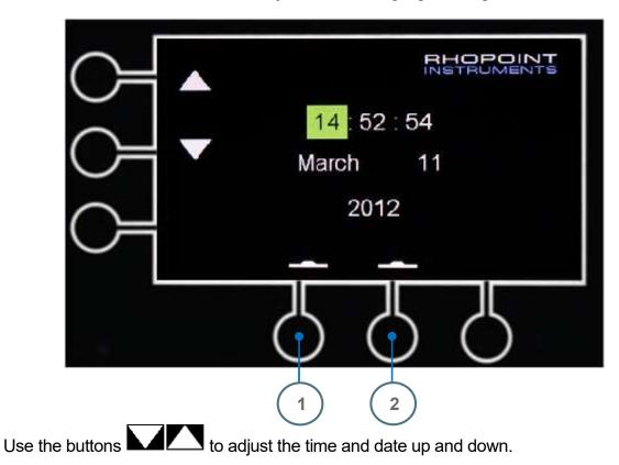
Pres Button 2 to adjust the next field. Once complete press button 1 to return to the main screen.
