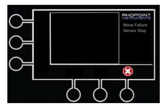
Press the red cross button *was* and the home button *will become active.* Remove any obstruction from the load cell and press the home button.
