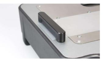
The sample size for the sled should be 63.5mm square. When measuring flexible samples the size can be 63.5x148mm and wrapped around the sled. The foam pad on the bottom will ensure a 63.5mm square contact area.
