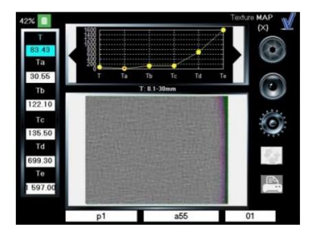
Provides a live view of the sample surface allowing the Optimap to be accurately positioned on the area of interest.
