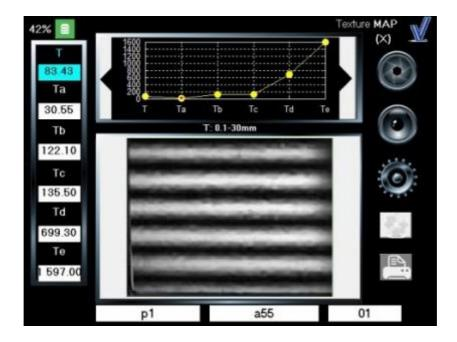
Projects a fringe pattern onto the surface in the Y direction. Useful for pre-measurement directional analysis of texture and / or defects.
