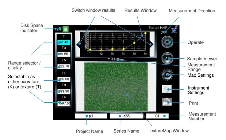
The touch sensitive icon based measurement screen provides operation and setup of the device.
