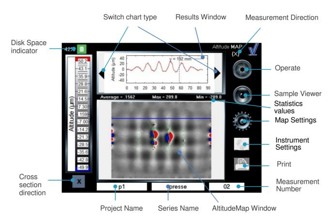
To the left of the altitude main screen a scale is displayed corresponding to the image displayed in the AltitudeMap window. The cross section direction button underneath the scale allows the switching of the cross section view, either X, Y or X/Y, that is displayed in the results window.
