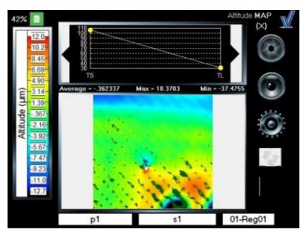
The Region feature is available for the Altitude/Curvature/Texture mode and dual/multi band and X, Y, X+Y directions. When a region is created the measurement number is renamed as 01-Reg01.
