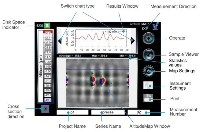
By double tapping the Texturemap window it allows full screen viewing of the sample surface –
