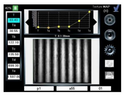
Projects a fringe pattern onto the surface in the X direction. Useful for pre - measurement directional analysis of texture and / or defects.
