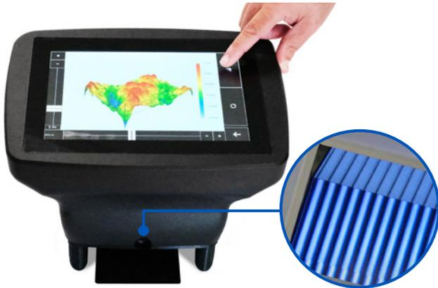
**Phase Measurement Deflectometry (PMD) is used to map surface topography**
