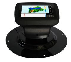
Its large measurement area ( $65 \times 54$ mm) and speed of operation (under 10 secs) provides rapid measurement with results that are more representative than those made with profilometers or other optical scanning instruments and can be reported in traceable SI units or other industry specific units.
