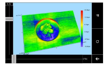
Cross sections can be created through the surface by touching the relevant point of interest on the displayed image and viewing the chart in the upper display.
