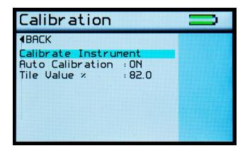
The Calibration Screen is used to setup the instrument calibration to the user's preference. Pressing the Up and Down buttons navigates through the options, pressing the Enter button selects that option.
