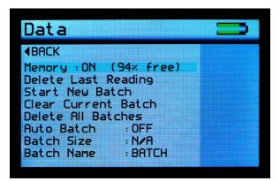
The Data Screen is similar in functionality to that of the menu screen but also allows the selection and setting of the Auto Batch size.
