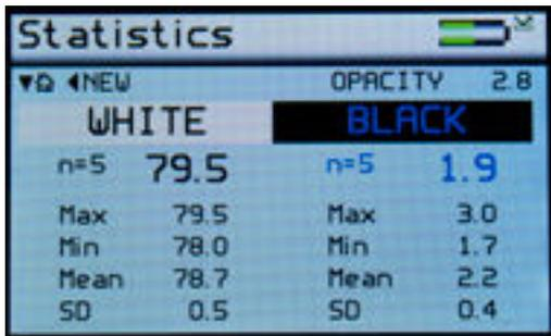
Measurements are made over a white substrate and then over a black substrate. Opacity is automatically calculated and displayed.
