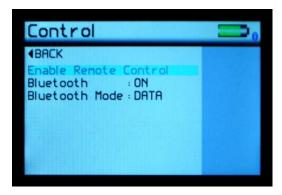
If the Bluetooth icon is not visible, enable it as detailed in Control Screen.
