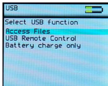
**Access Files** – Allows access to measurement and configuration files on the instrument. The instrument appears as a USB drive named IQ-METER. When selected the display on the instrument shows a USB memory key as shown below.
