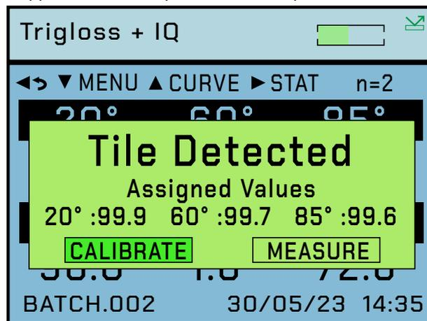
Two options are available: either to "Calibrate" the instrument on the calibration standard before making the measurement or to "Measure" without performing a calibration. Press the **Left/ Right** and **Enter** buttons on the keypad to select the required option.
