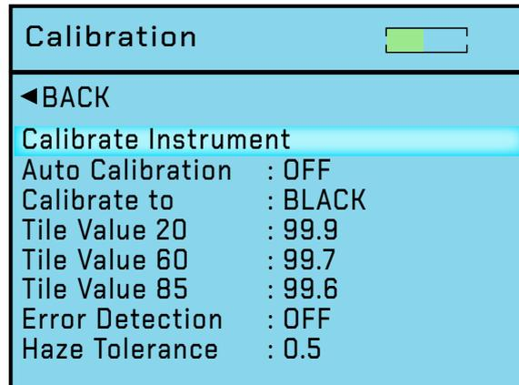
The Calibration Screen is used to setup the instrument calibration to the user's preference. Press the Up / Down buttons to navigate through the options, press the Enter button to select the option required. Options in the Calibration screen are: -
