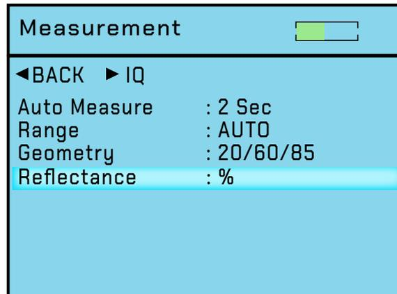
The Measurement Screen is used to configure the instruments measurement parameters to the user's preference. Press the **Up / Down** buttons to navigate through the options, press the Enter button to select the option required.
