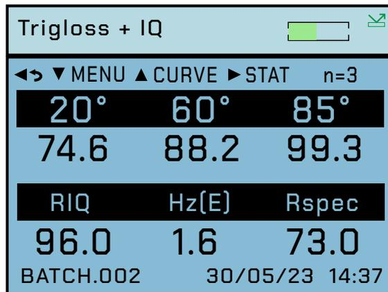
In the Home screen press the **Up** button to access the Reflectance curve screen. The goniophotometric profile and data for the last 20° measurement is displayed.
