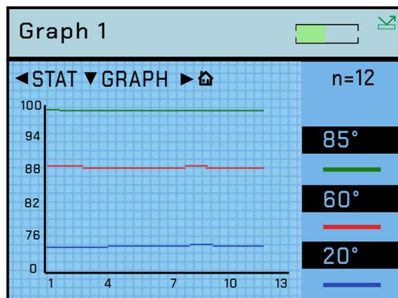
Measurements can be taken whilst in this screen and the graph will be updated after each reading.
