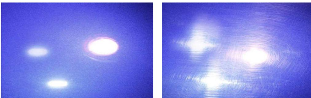
Haze is an important measure for highly polished metals and is often associated with polishing marks and machining direction.
