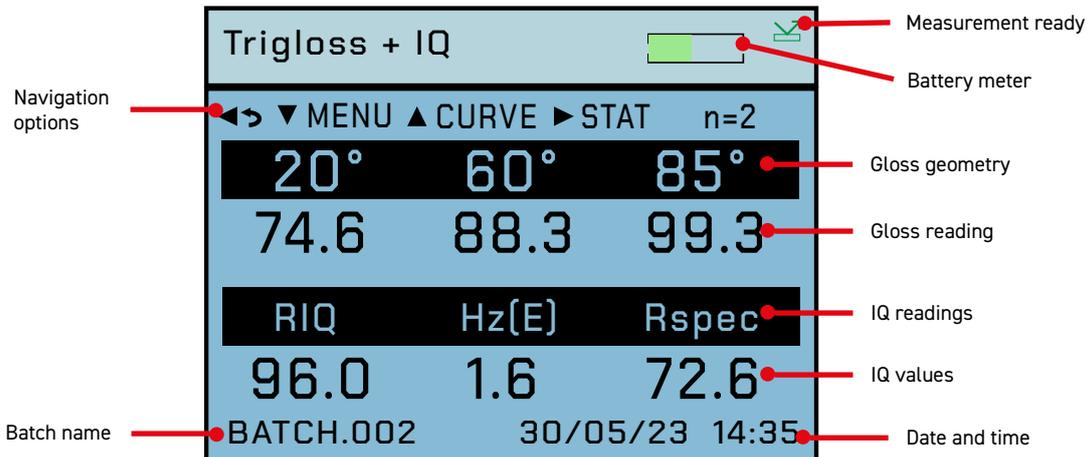
In this mode, measurements can be made by simply pressing the **Operate** button on the instrument's keypad.
