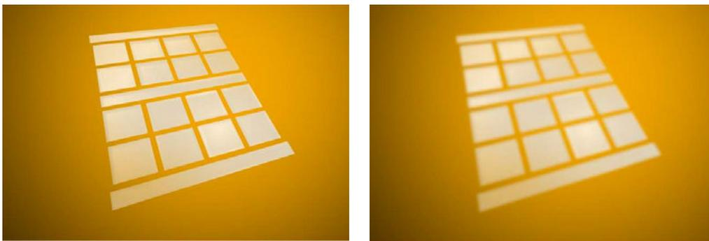
When viewing the reflection of a strong light source in a surface with high haze the image "blooms" and has a bright halo around it.
