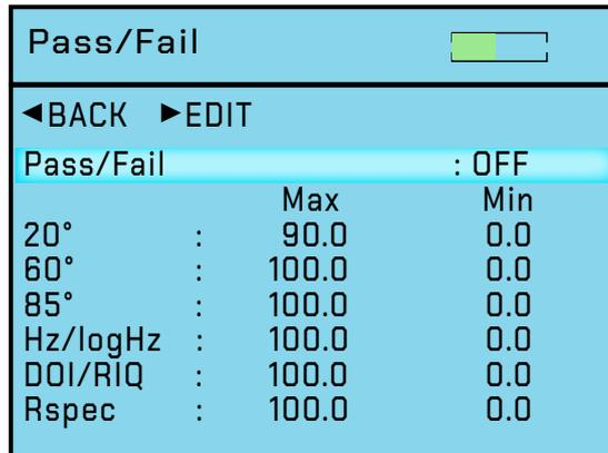
The **Pass/Fail** setup screen is used to enable/disable on-screen pass/fail indication and set min / max tolerancing. Press the down key to select the Pass/Fail option and press the center button to toggle the feature ON or OFF.
