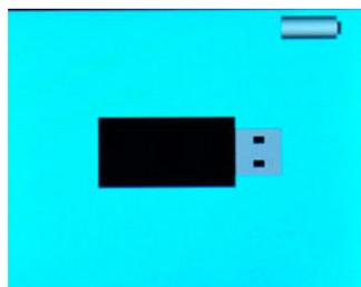
**USB Remote Control** - Allows control of the IQ remotely by sending ASCII commands from a computer or PLC. In this mode the instrument displays "REMOTE CONTROL ACTIVE" on the main measurement screen.
