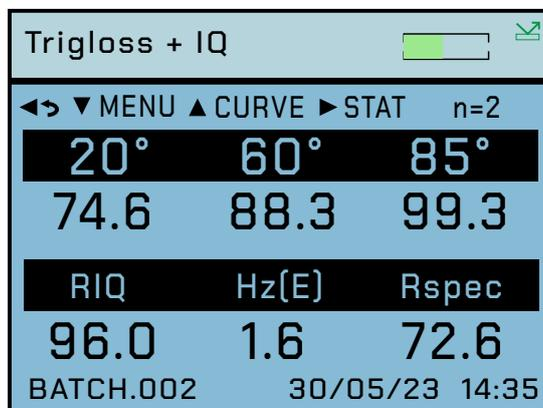
**Haze Compensation** – Selects either ON or OFF. Haze compensation is not available when ASTM D4039 is selected. With haze compensation selected to ON a (C) identifier will be displayed additionally next to the Hz parameter. Further details of Haze Compensation can be found in the Appearance Theory section of this manual.
