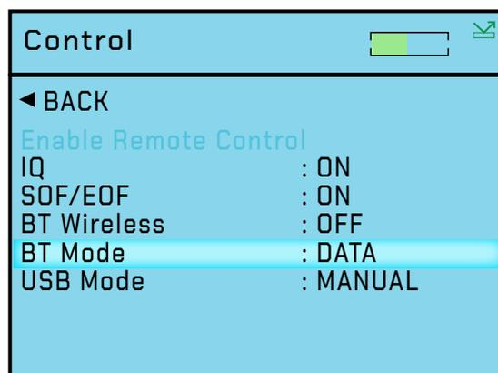
The Control Screen is used to configure the instruments Bluetooth parameters to the user's preference. Press the **Up / Down** buttons to navigate through the options, press the Enter button to select the option required.
