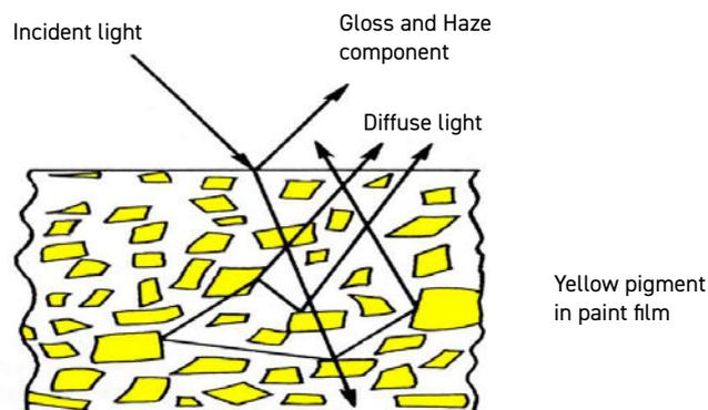
The Rhopoint IQ compensates for reflection from within the coating for highly reflective pigments, metallic coatings and speciality pigments, allowing the haze of any painted surface to be measured.
