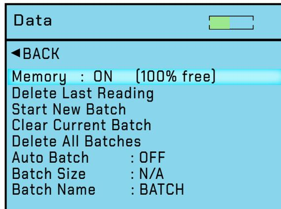
The Data Screen is similar in functionality to that of the menu screen but also allows the selection and setting of the Auto Batch size.
