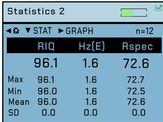
Press the **Right** button in the statistics screen to display the graph screen; this screen displays a trend graph of IQ measurement data. Press the **Down** button to sequentially display IQ data either all together or individually.
