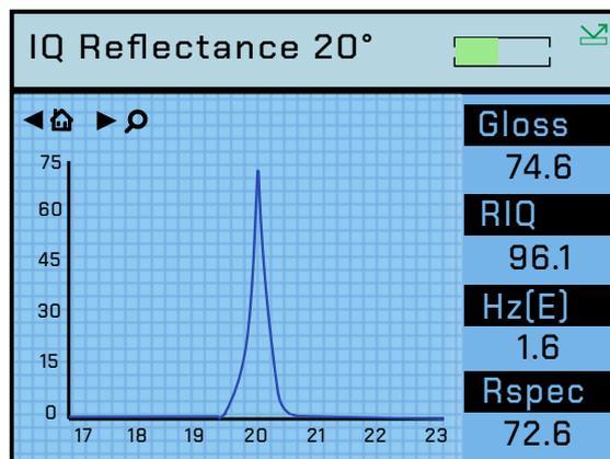
Measurements can be taken whilst in this screen and the display will update. Press the Right button to zoom in, the Y axis will auto-scale to fit the reflectance curve data. Press the Left button to return to the Home screen.
