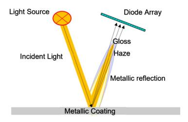
The Rhopoint IQ captures compensation information from a region adjacent to the haze measurement angle, this means it can be used on metallic coatings which reflect light directionally
