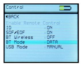
The Control Screen is used to configure the instruments Bluetooth parameters to the user's preference. Press the Up / Down buttons to navigate through the options, press the Enter button to select the option required.
