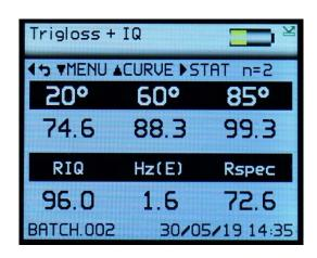
Haze Compensation – Selects either ON or OFF. Haze compensation is not available when ASTM D4039 is selected. With haze compensation selected to ON a (C) identifier will be displayed additionally next to the Hz parameter. Further details of Haze Compensation can be found in the Appearance Theory section of this manual.
