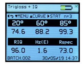
In the Home screen press the Up (3) button to access the Reflectance curve screen. The goniophotometric profile and data for the last 20° measurement is displayed.
