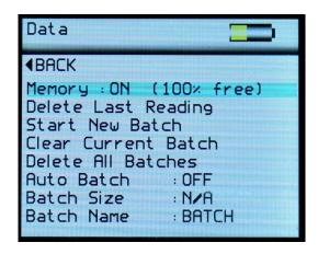
The Data Screen is similar in functionality to that of the menu screen but also allows the selection and setting of the Auto Batch size.
