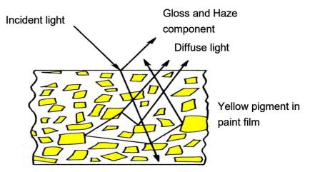
The Rhopoint IQ compensates for reflection from within the coating for highly reflective pigments, metallic coatings and speciality pigments, allowing the haze of any painted surface to be measured.
