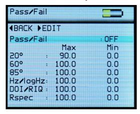
The Pass/Fail setup screen is used to enable/disable on-screen pass/fail indication and set min / max tolerancing. Press the down key to select the Pass/Fail option and press the center button to toggle the feature ON or OFF.
