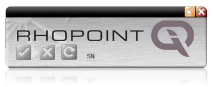
5. The buttons are greyed out while the DATA widget searches for SWITCHED ON IQ(s) that have been PAIRED to the PC.
