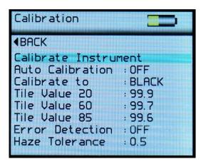
The Calibration Screen is used to setup the instrument calibration to the user's preference. Press the Up / Down buttons to navigate through the options, press the Enter button to select the option required. Options in the Calibration screen are: -
