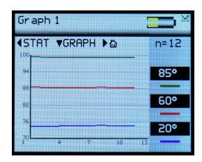
Measurements can be taken whilst in this screen and the graph will be updated after each reading.
