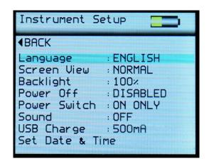
The Instrument Setup screen is used to configure the instruments basic operating environment to the user's preference. Press the Up / Down to buttons navigate through the options, press the Enter button to select the option required.
