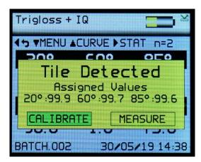
Two options are available: either to "Calibrate" the instrument on the calibration standard before making the measurement or to "Measure" without performing a calibration. Press the Left/ Right (3) and Enter (4) buttons on the keypad to select the required option.
