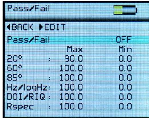
The Pass/Fail setup screen is used to enable/disable on-screen pass/fail indication and set min / max tolerancing. Press the down key to select the Pass/Fail option and press the center button to toggle the feature ON or OFF.
