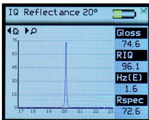
Measurements can be taken whilst in this screen and the display will update. Press the Right button to zoom in, the Y axis will auto-scale to fit the reflectance curve data. Press the Left button to return to the Home screen.
