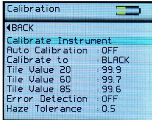
The Calibration Screen is used to setup the instrument calibration to the user's preference. Press the Up / Down buttons to navigate through the options, press the Enter button to select the option required. Options in the Calibration screen are: -
