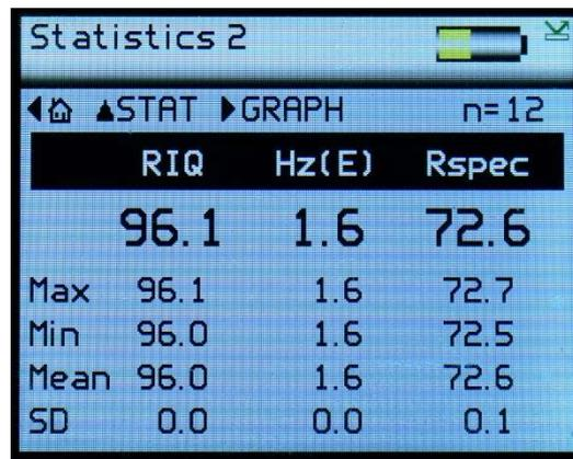
Press the Right button in the statistics screen to display the graph screen; this screen displays a trend graph of IQ measurement data. Press the Down button to sequentially display IQ data either all together or individually.
