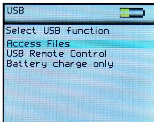
Access Files – Allows access to measurement and configuration files on the instrument. The instrument appears as a USB drive named IQ-METER. When selected the display on the instrument shows a USB memory key as shown below –
