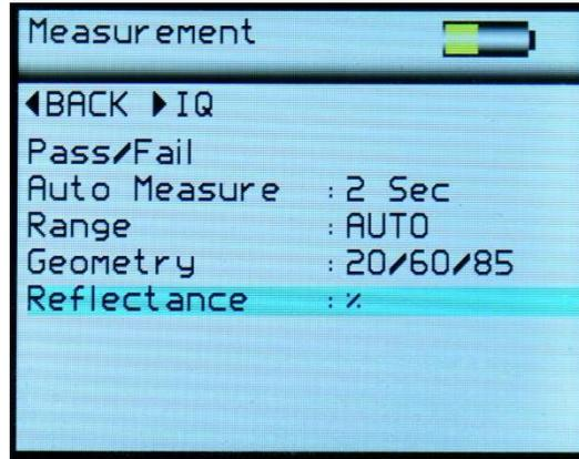
The Measurement Screen is used to configure the instruments measurement parameters to the user's preference. Press the Up / Down buttons to navigate through the options, press the Enter button to select the option required.
