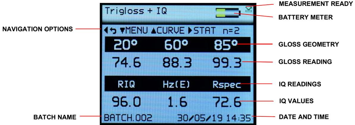
In this mode, measurements can be made by simply pressing the operate button (4) on the instrument's keypad.
