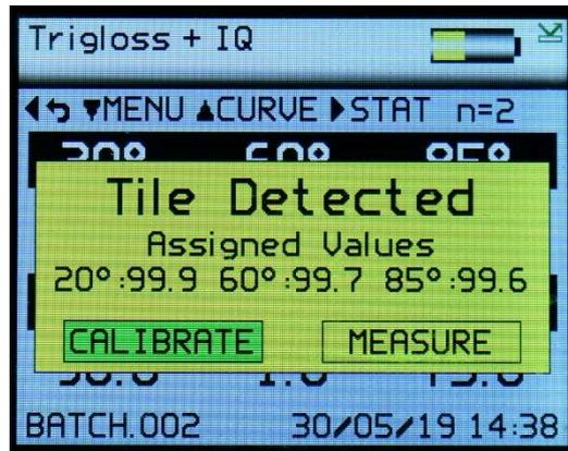
Two options are available: either to "Calibrate" the instrument on the calibration standard before making the measurement or to "Measure" without performing a calibration. Press the Left/ Right (3) and Enter (4) buttons on the keypad to select the required option.
