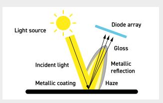
The IQ Flex 20-S captures compensation information from a region adjacent to the haze measurement angle. This means it can be used on metallic coatings which reflect light.
