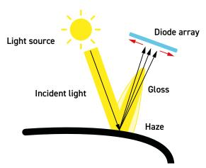
The IQ Flex 20-S automatically adjusts for non-flat surfaces by sensing the reflected peak and virtually adjusting the position of the sensor.
