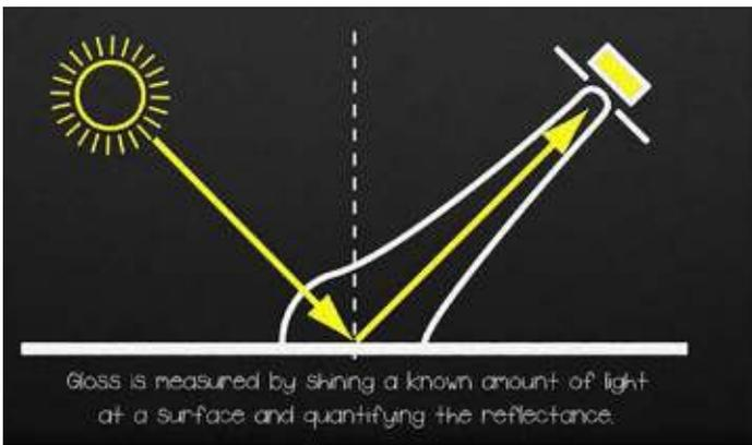
The angle of the light and the method by which the reflectance is measured are determined by the surface material and which aspect of the surface appearance is to be measured.
