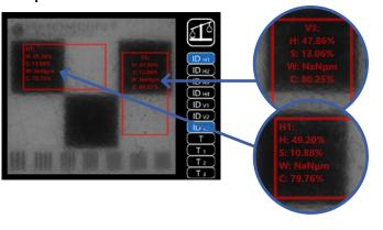
Surface waviness in not measurable due to high orange peel effect
