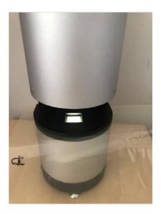
STEP 2: The samples were mounted onto the surface roughness and small parts ASTM (8mm) adaptor on the measurement graticule to obtain results compatible with ASTM D1003.
