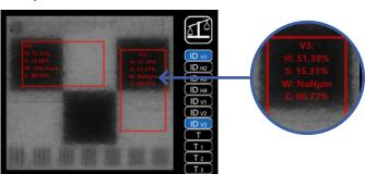
Surface waviness in vertical direction not measurable due to high orange peel effect
