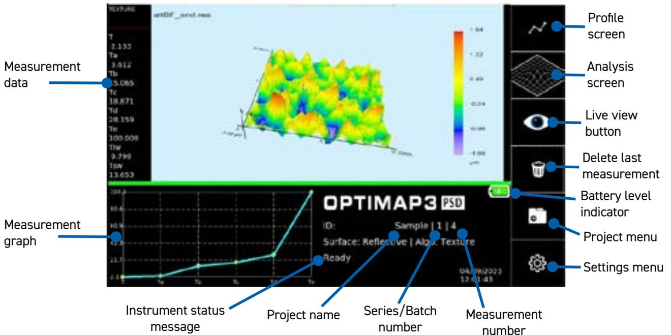
The touch sensitive icon-based measurement screen provides operation and setup of the device. By pressing each of the icons or active areas shown on the screen the instrument responds in a different way according to the function.
