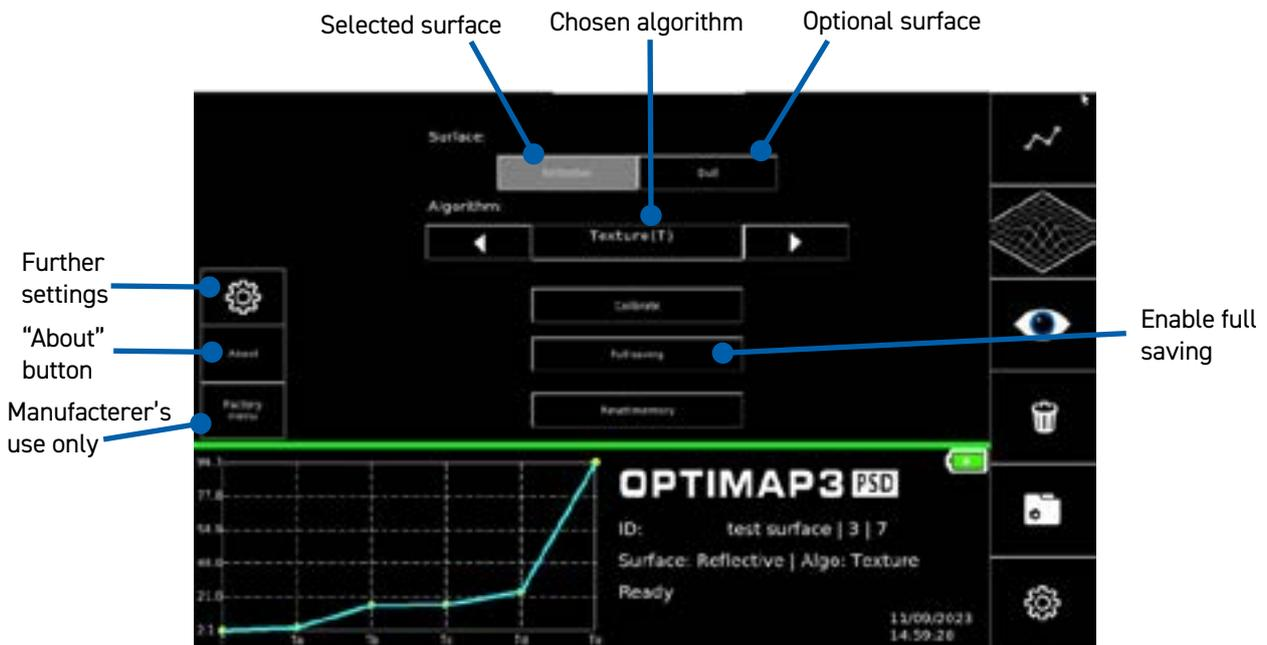
To allow the measurement of a wide range of surface finishes the Optimap has two optical configurations (models) available for selection – Reflective and Dull.
