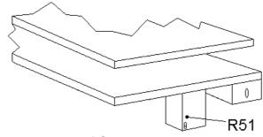
Fig. 7.3.3. Location of Calibration screws on bottom PCB.
