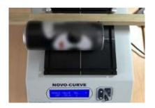
**STEP 1:** Location jigging posts and a long, wooden spacer were used on the instruments measuring platen to centralise the can onto the aperture to ensure repeatable results were made each time.
