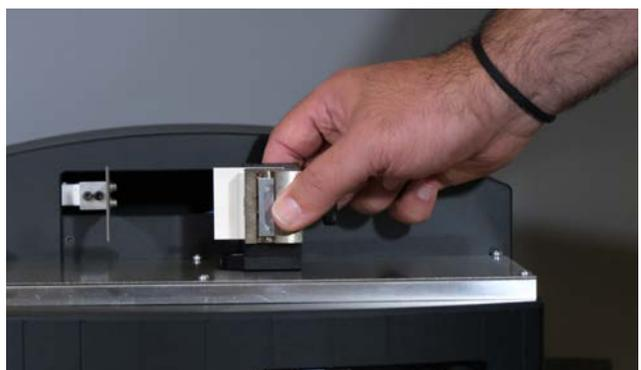
**Rounded corner crease resistance:** Rounded corner creases can be tested on the CFA (requires additional jaw).
