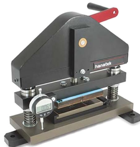
Prepares individual crease and stiffness samples. Suitable for low-medium volume testing.
