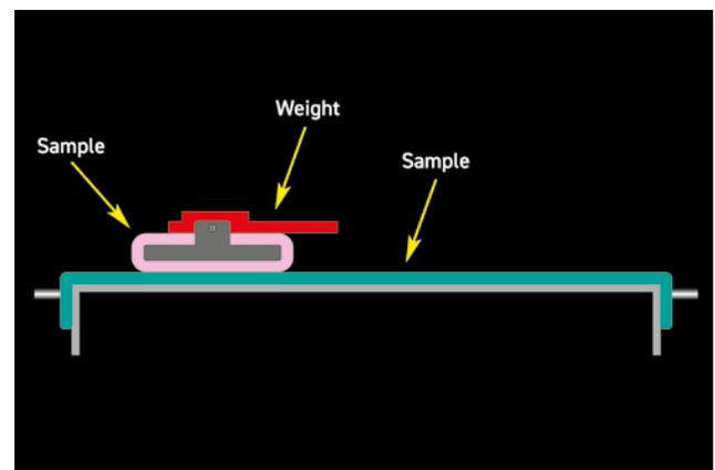
In practical terms, the static slip relates to the force required to get two resting surfaces moving, dynamic slip is the smaller force that is required to keep the surfaces moving once this initial "inertia" is overcome. These values are expressed as ratios and do not have units, they are usually quoted as a decimal value between 0 and 1.
