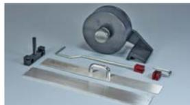
Peel test attachments
