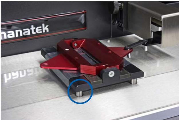
Sled is positioned on lift pins
