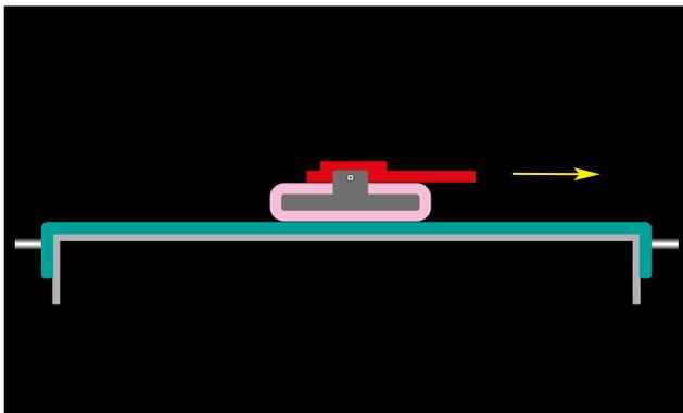
Original slip testing instruments were converted tensile testers that used a cord to pull the sample. The use of a cord has now been removed from most friction measurement standards due to the uncertainty added by its own elasticity and problems with sample positioning.
