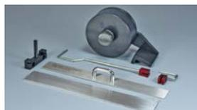
Peel test attachments
