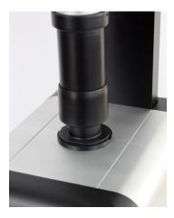
Take a reading on the checking standard by pressing the tick icon and compare the result with its assigned value. The value must match the assigned value within the tolerances printed on the label.
