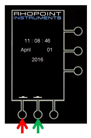
Press the button marked with a green arrow to start adjusting the time and date.
