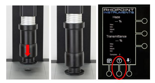
The measuring icon (tick) will now be displayed on the screen (see below). The instrument is now ready to take readings.
