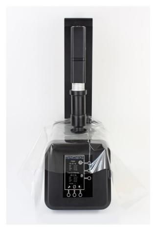
To take a reading, press the tick button. The instrument will operate and the results will be displayed on the screen. If a record of each reading is required, press the export button to send the result to a data stick or printer. See the export section of this manual for more details. Continue taking readings by pressing the tick button. Statistics are updated with each measurement. To reset the statistics delete the readings from the instrument memory (see below).
