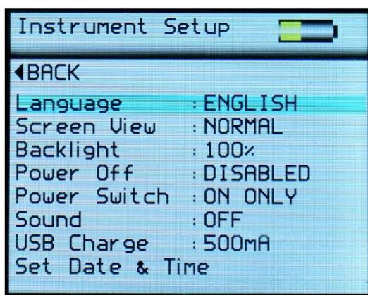
The Instrument Setup screen is used to configure the instruments basic operating environment to the user's preference. Press the Up / Down to buttons navigate through the options, press the Enter button to select the option required.
