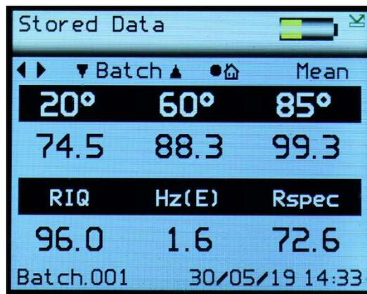
When Memory is set to ON (as detailed later in the Menu Screen section of this manual) measurements can be recalled and displayed from any batch stored in the IQ memory.
