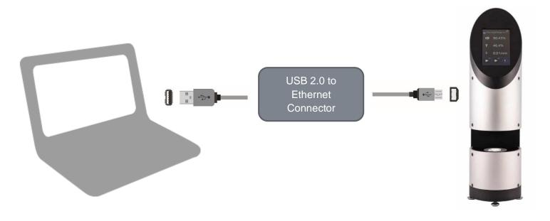
**LAN Connection**: the software can operate multiple instruments which are connected to a local network.
