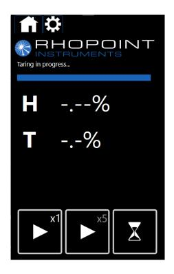
Once taring is complete measurement buttons are available and the instrument is ready for use.
