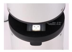
The standard is held in place by magnets; ensure that the back of the standard is aligned with the edges of the instrument body.
