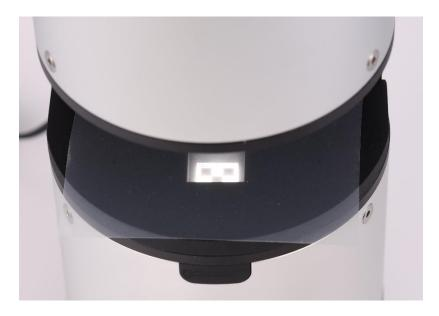
Measuring with the ASTM haze spacer in place is often the default method for many applications.
