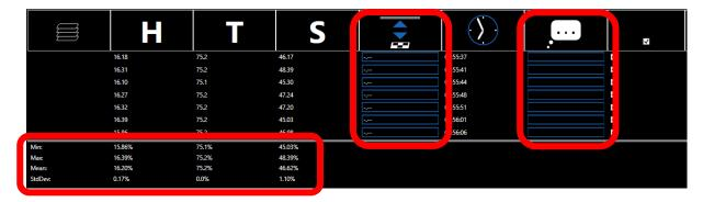
**Add measurement distance-** To add a measurement distance to the measurement data the distance text box should be used.
