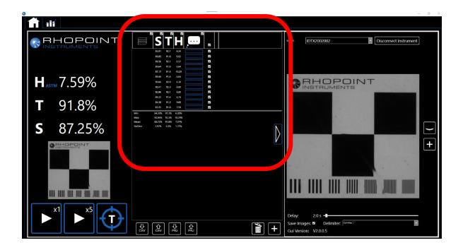
The center Panel of the software contains the results for all measurements taken in the current batch. The bottom section contains statistics for all the results listed in the table.
