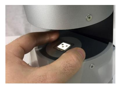
For fast easy manipulation high clarity samples with low distance dependency can be manually held and moved.
