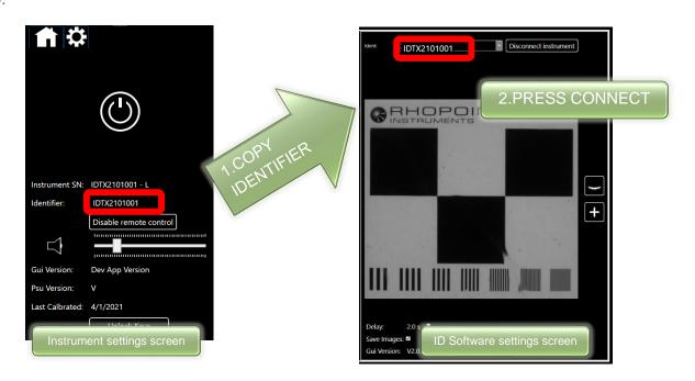
NOTE: If the instrument is connected via a LAN the text .local may need to be added directly after the instrument serial number (no space)
