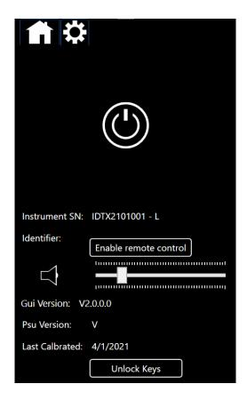
To power off the instrument press & hold the power icon.
