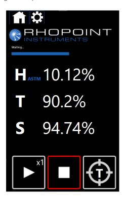
The instrument introduces a delay before starting the first measurement and between readings- this allows the user time to manipulate the sample. To finish an ∞ batch press the stop button, the instrument will report the statistical analysis for the measured samples.
