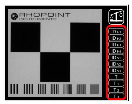
The on instrument T value is calculated using the transmitted light through all black and white areas- this area can be viewed by toggling the T button.
